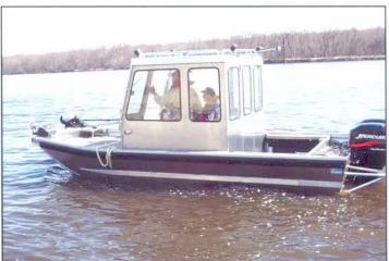
The overall boat configuration is tailored to your application through a variety of options such as length, width, and bottom profile. The hull's floor design allows for ribless interior sidewalls. Minimum .190 marine grade welded aluminum construction. All features provide a durable and dependable workboat hull.
