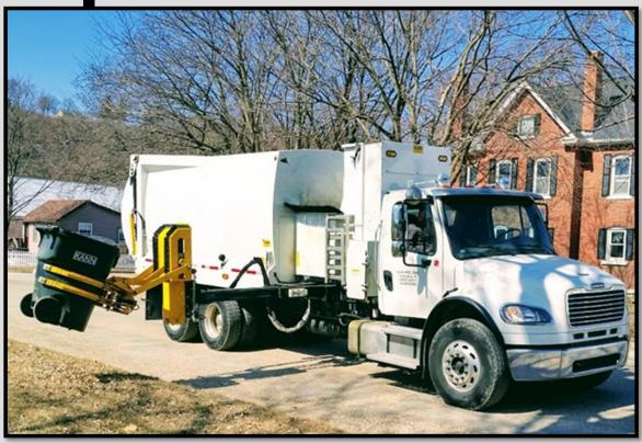
The KANN Automated Two Compartment Split Side Loader comes in six body sizes ranging from 18 to 30 cubic yards, with an arm reach of up to 10 feet, loading cycle of 8 seconds and capable of up to 850 lbs/yd³ to maximize payloads!
